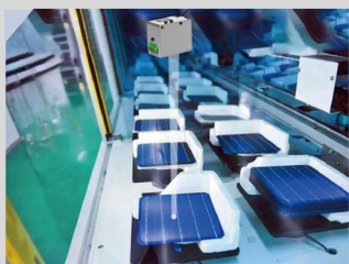
Detection of wafer size change Sensors used: LA-W500N
